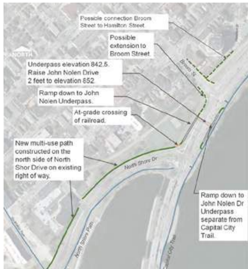
Figure D.16 North Shore Drive-Long Term Solution (Blair Street Corridor Study Report)
