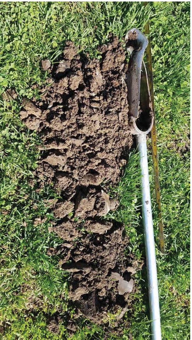
The soils at this sample point appears to be fill material.
