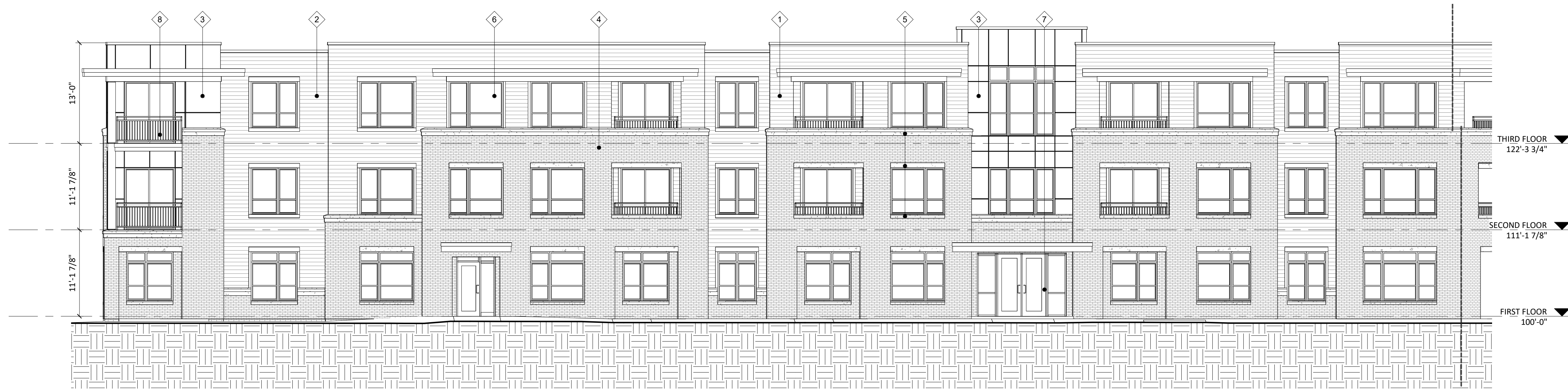
1 ELEVATION - NORTH WEST A201 1/8" = 1'-0"
