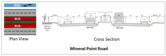
Figure 10.0-2 Mineral Point Road Running Way
