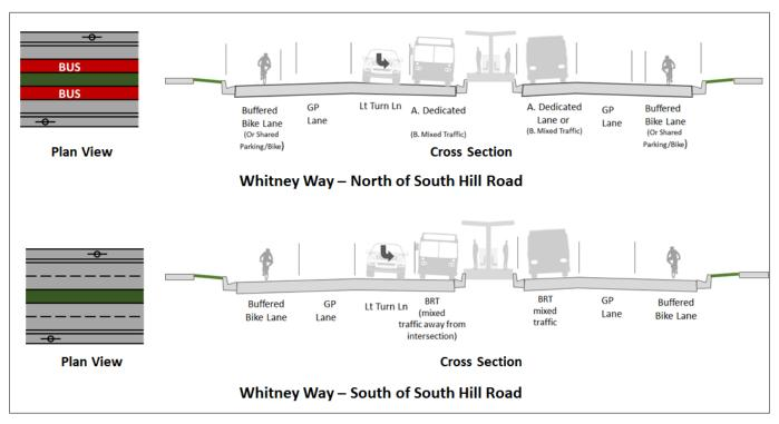
Figure 10.0-3 E-W BRT Running Way
