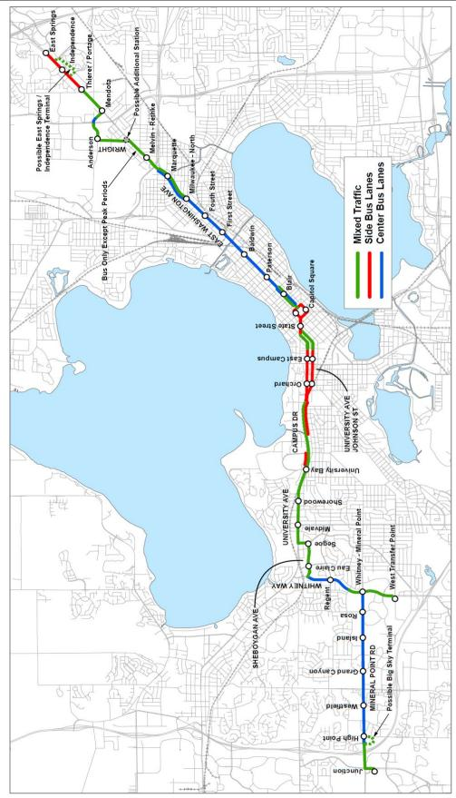
Figure 10.0-1 E-W BRT Running Way
