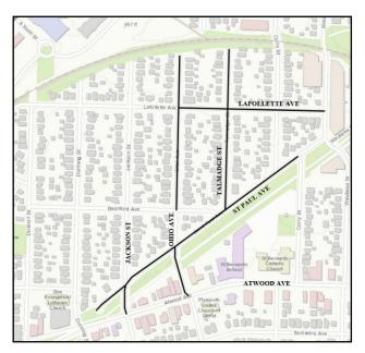
Ohio Ave (between Atwood and St Paul) will be reconstructed to a 20-ft wide street (existing width is 28-ft) and converted to a 1-way with northbound-only traffic and parking only on the east-side of the street, thus removing parking on the west-side and widening the concrete terrace in front of the Ohio Tavern. The existing concrete terrace on the east-side of the street will be replaced with grass.
