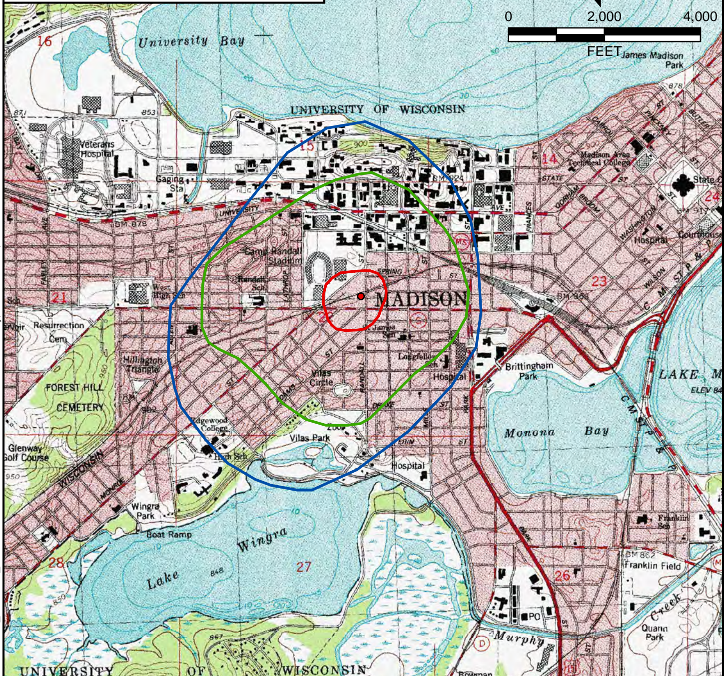
FIGURE 3-1 5, 50, 100 YEAR T.O.T. Z.O.C.s ASSUMING PROJECTED 2030 PUMPING RATE UNIT WELL 27 MADISON, WISCONSIN
