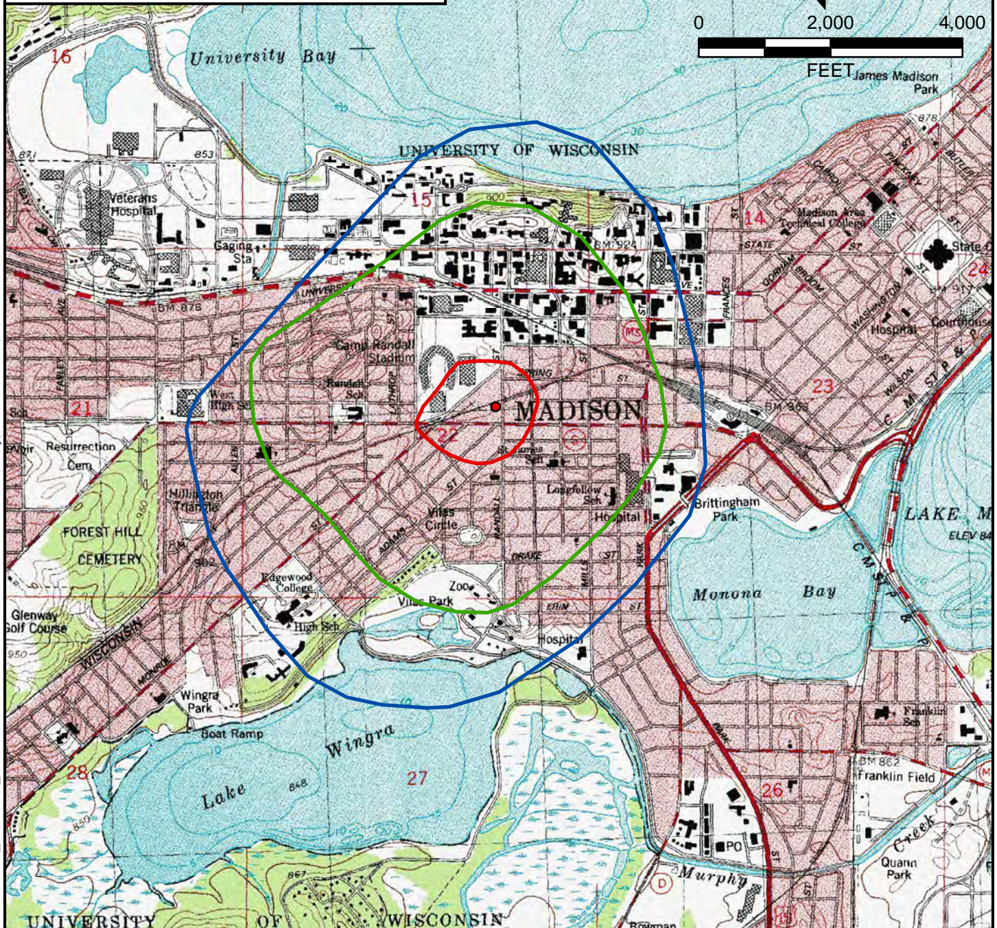
FIGURE 3-4 5, 50, 100 YEAR T.O.T. Z.O.C.s ASSUMING PUMPING AT AVG RATE DURING MAX YEAR UNIT WELL 27 MADISON, WISCONSIN
