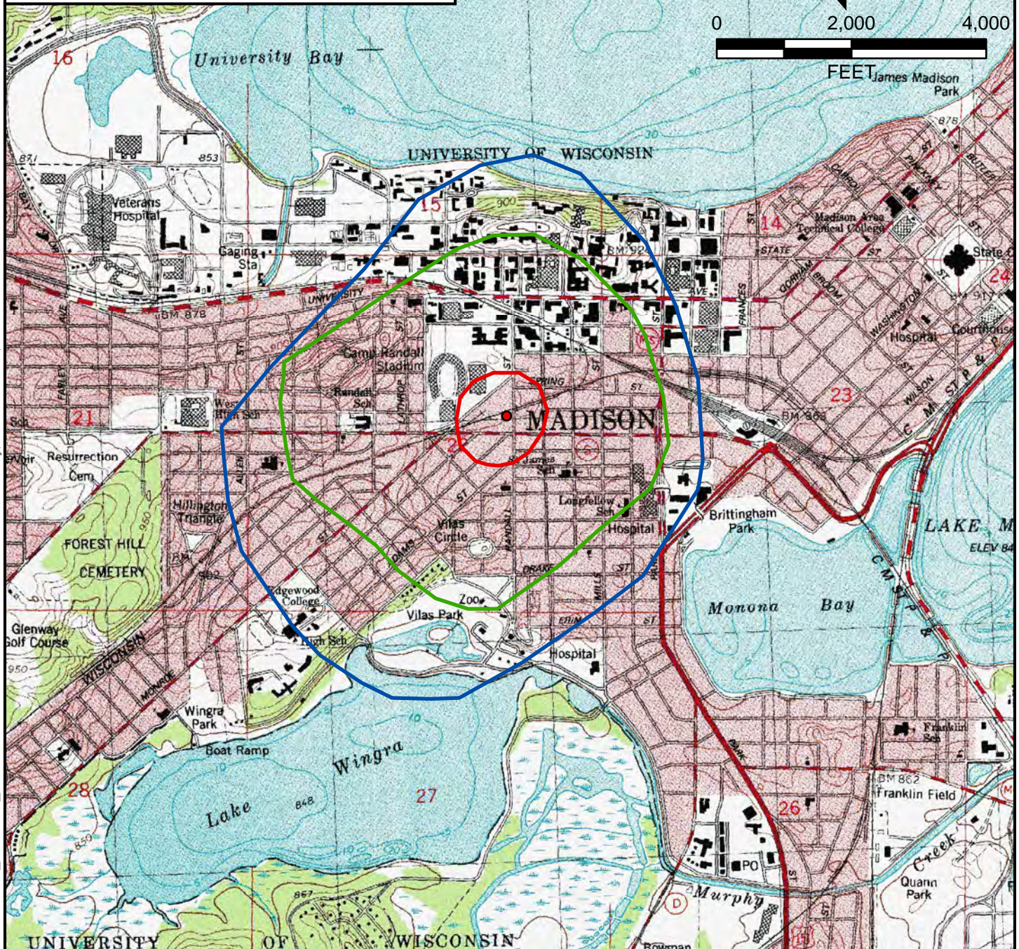
FIGURE 3-2 5, 50, 100 YEAR T.O.T. Z.O.C.s ASSUMING 50 PERCENT CAPACITY PUMPING RATE UNIT WELL 27
