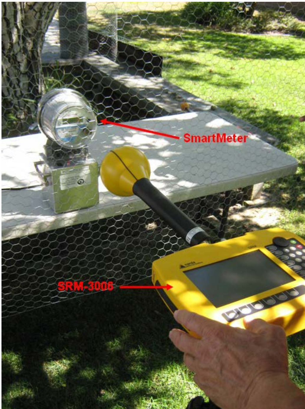
Figure 10-1 Measurement setup to determine the insertion loss presented by a conductive mesh (chicken wire in this case).
