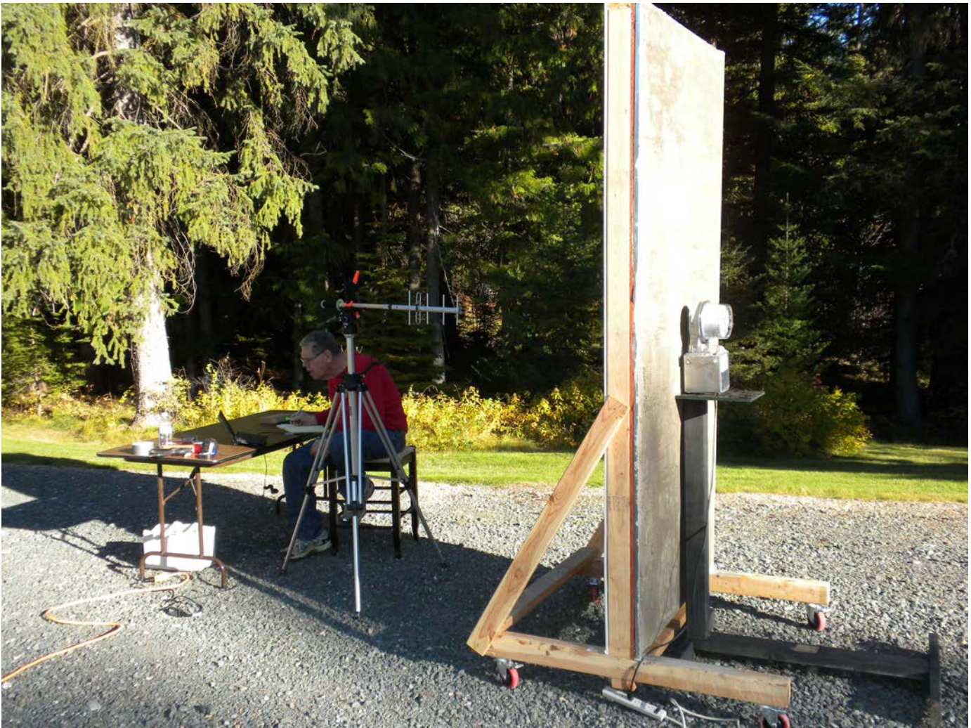
Figure 10-4 Measurement setup for determining insertion loss of simulate stucco wall shown with the 900 MHz yagi antenna.
