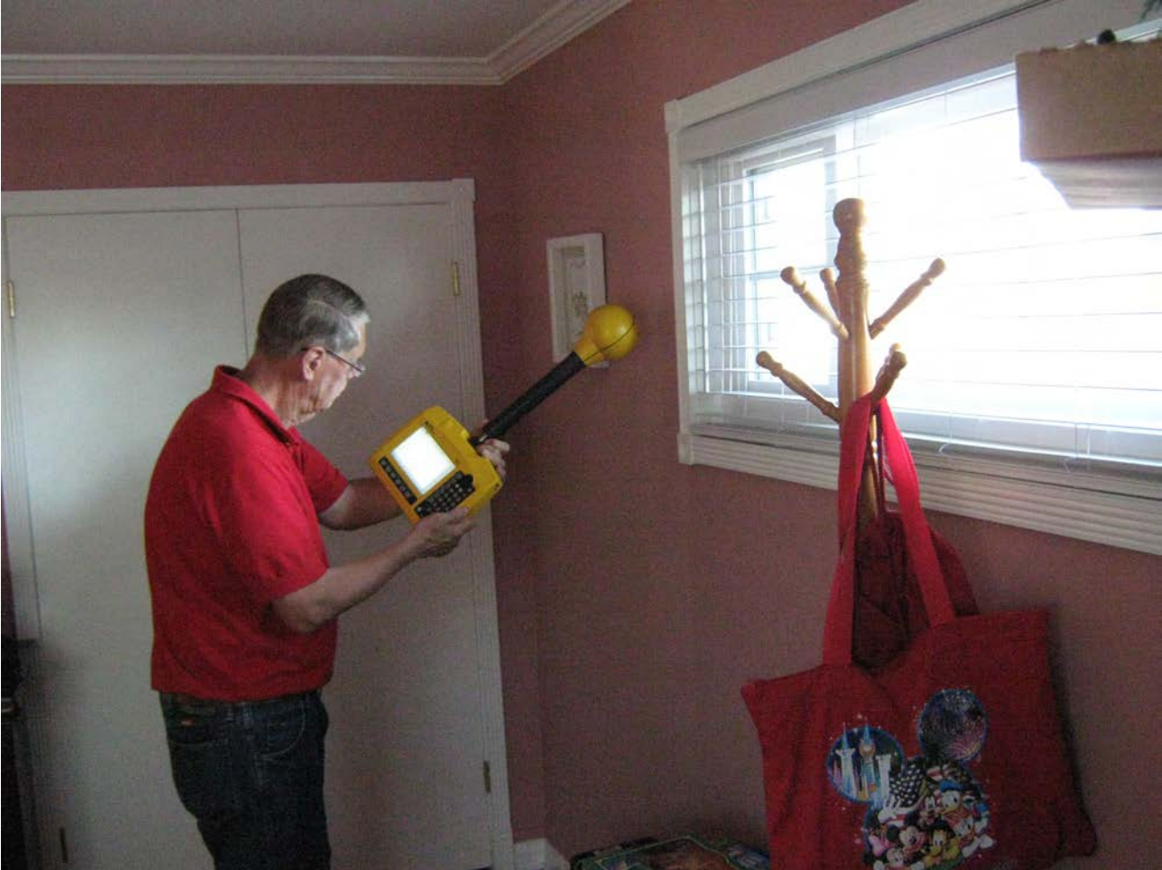
Figure 9-15 Interior residential measurements included measurements on the opposite side of the wall where the Smart Meter was installed at the home.
