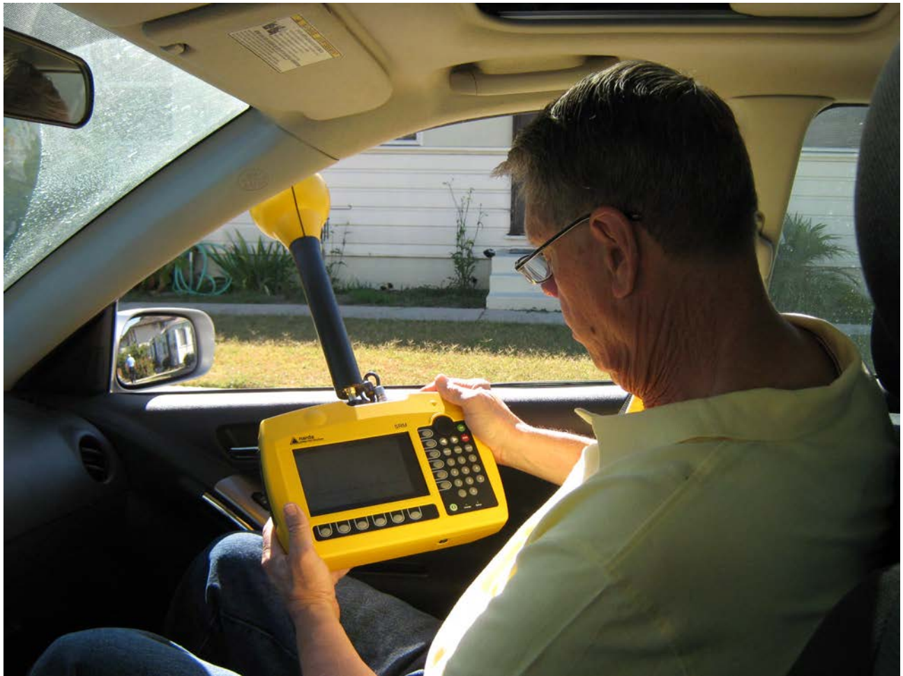
Figure 9-26 Conducting a "driving survey" of a Smart Meter deployed neighborhood.
