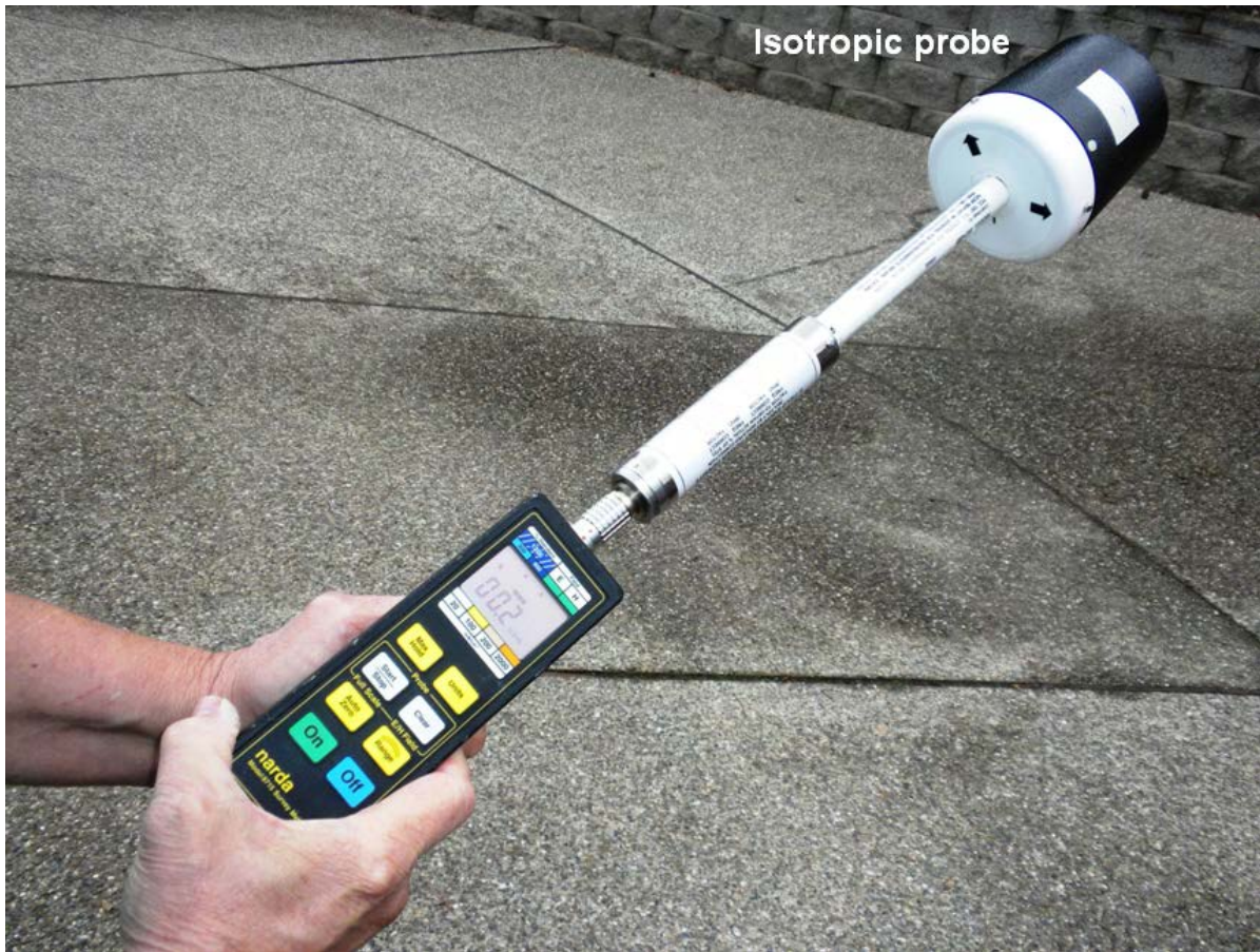
Figure 7-4 Frequency shaped, isotropic, electric field probe and meter (Narda B8742D and Narda 8715 meter).
