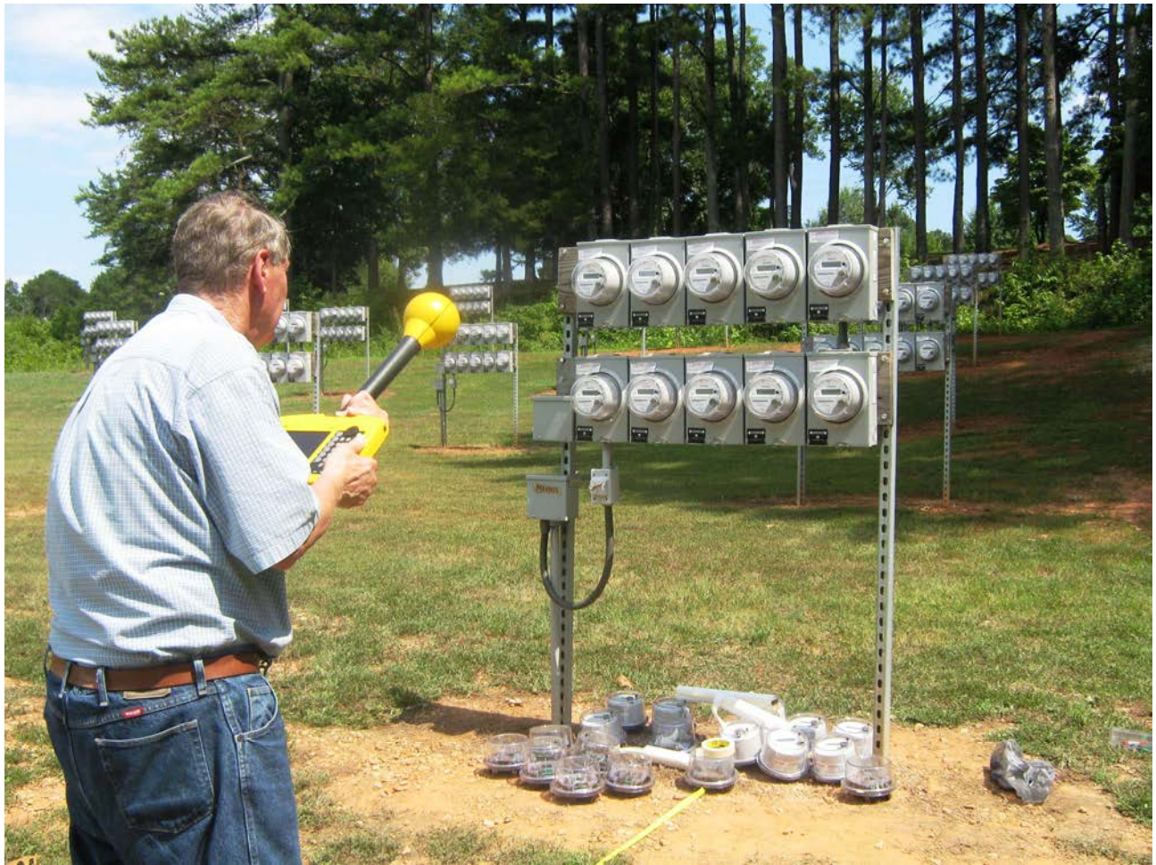
Figure 9-7 Using the Narda SRM-3006 to measure aggregate RF fields near a rack of ten meters programmed for fixed frequency, continuous transmission in the meter farm.
