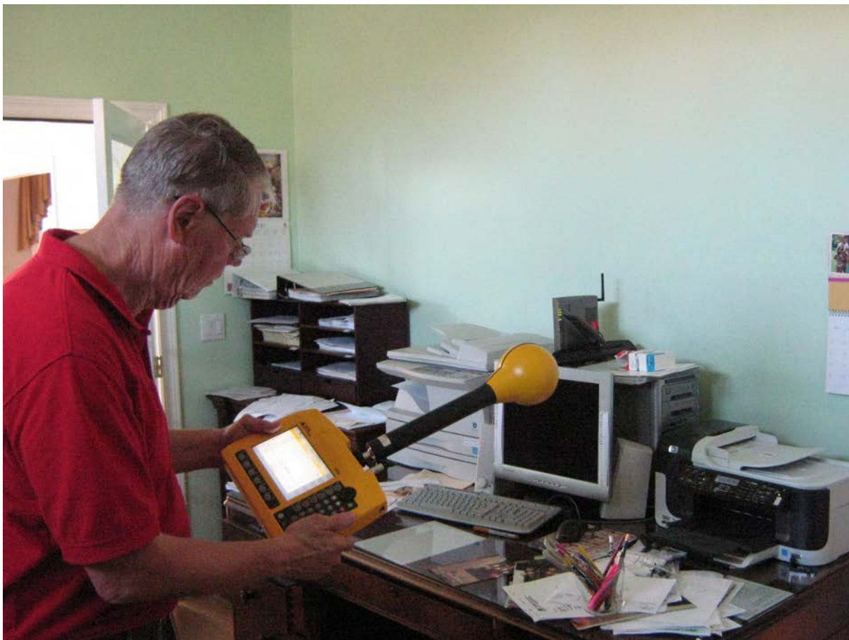
Figure 9-20 Measured RF fields inside residence B, similar to residence A, tended to be predominated by signals produced by wireless routers used for Internet connectivity throughout the home.
