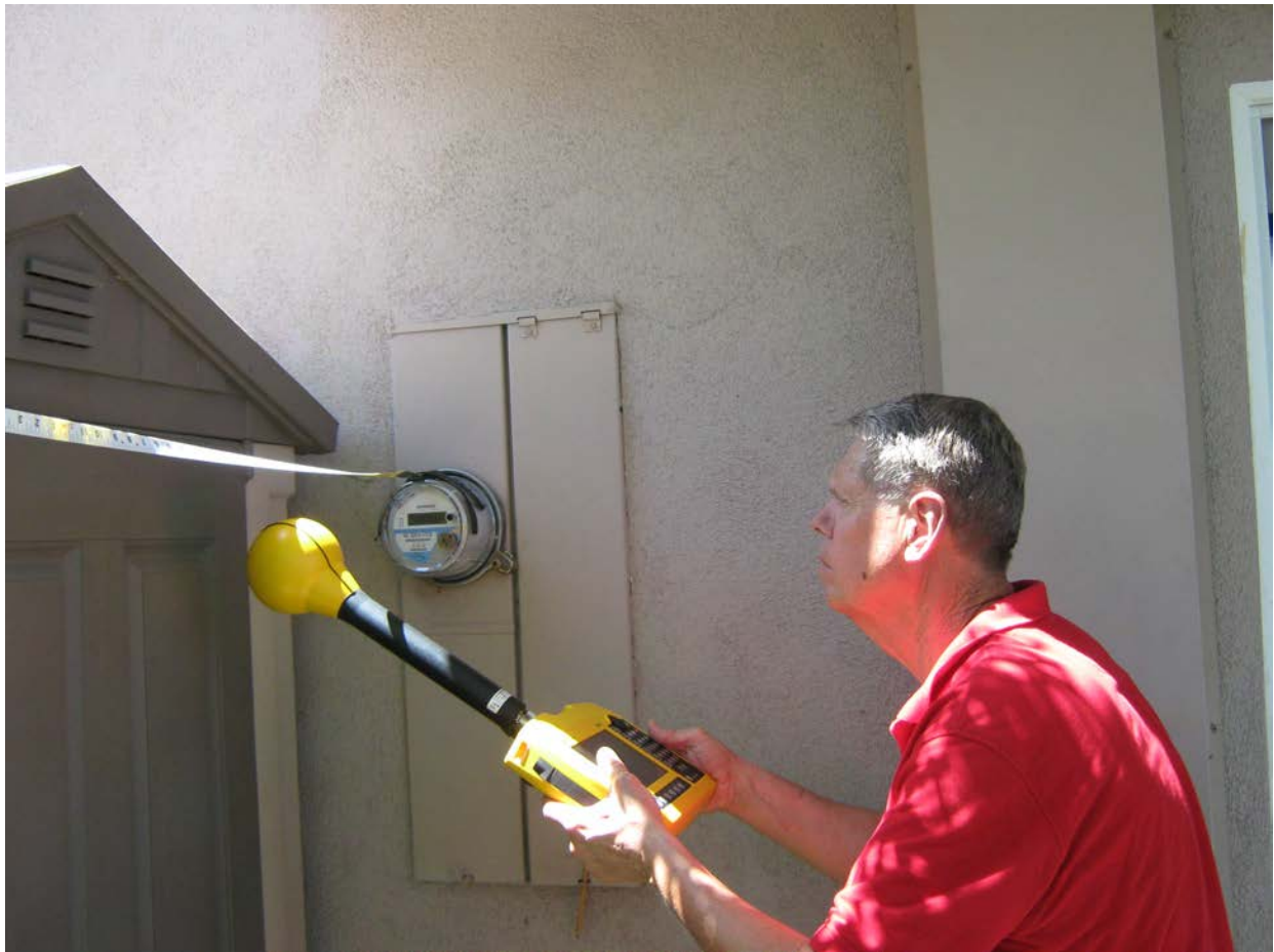
Figure 9-19 Performing a planar scan of RF fields adjacent to a Smart Meter at residence B.
