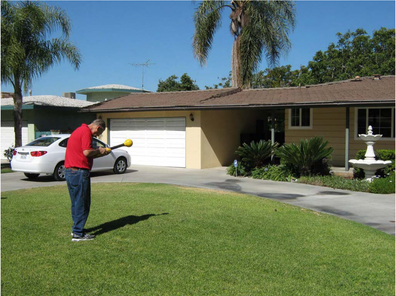
Figure 9-16 Residential measurements at residence A included both outdoors and indoors measurements of RF fields in both the 900 MHz and 2.4 GHz bands.
