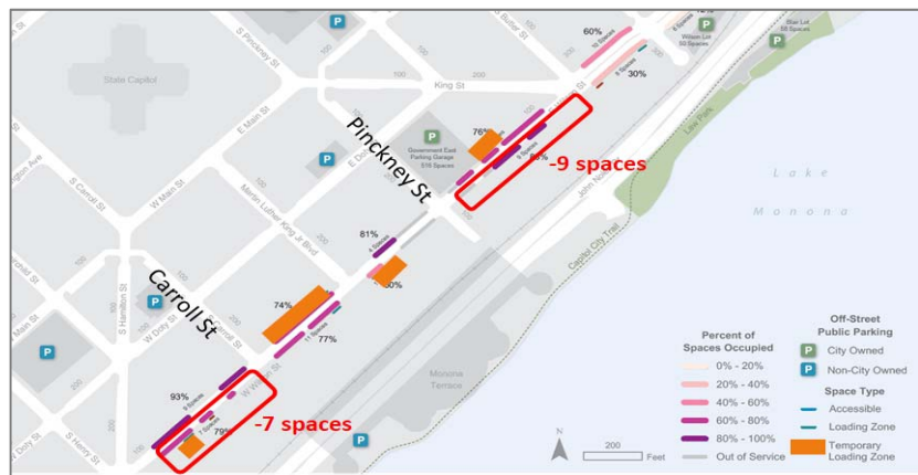
Figure 2.3-8 Parking eliminated with two-way protected cycle track
